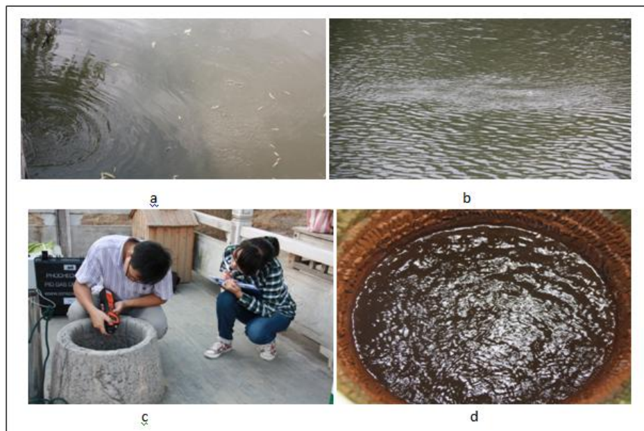
Fig. 15 bubbling phenomenon in "boiling well" and lakes and ponds in Danyang City, Jiangsu Province a. "bubble" in the lake five meters away from the boiling well; b. "bubbles" in ponds 20 meters away from the boiling well; c. Measurement of total volatile organic compounds in boiling well 1; d. bubbling phenomenon in boiling well 2
